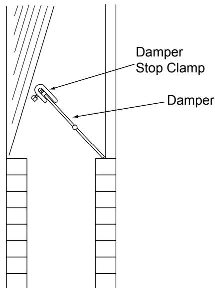
Figure 8 Damper Stop Clamp
