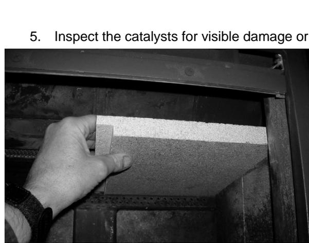
**Figure 18 (cont.) - Removing/Replacing the Baffle for Inspection**
