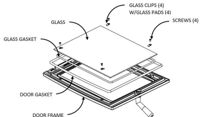
Figure 22: Front Door assembly
