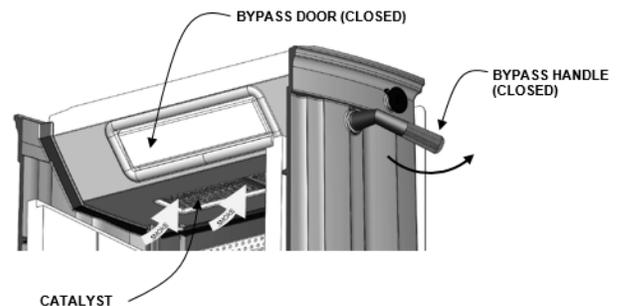
Figure 12 – Bypass Closed
